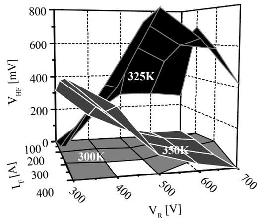
Figure 12: RF sensor voltage dependence for  $R_G=15\Omega$
