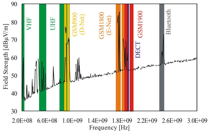
Figure 7: EMC measurement of environment
