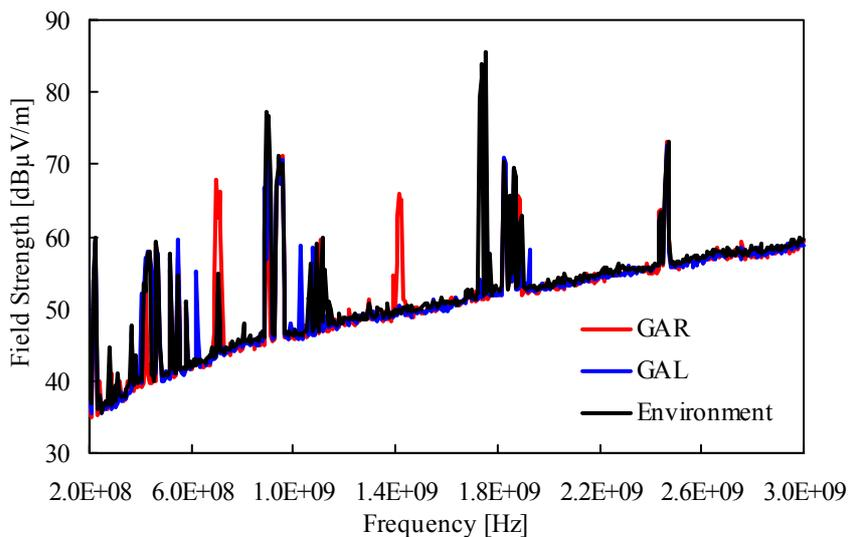
Figure 10: EMC measurement of GAR (pett) and GAL (no pett) in comparison with environment
