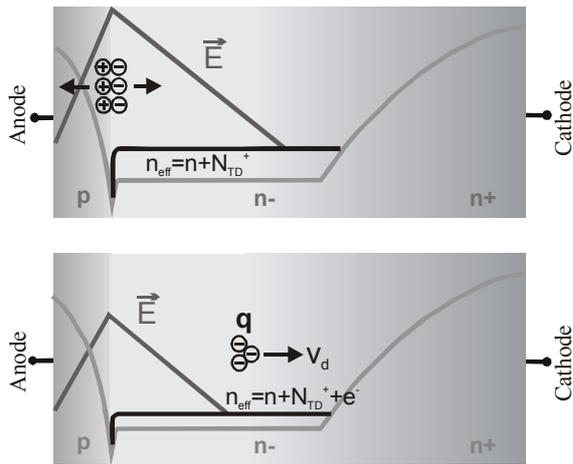
Figure 3: Origin of dynamic impatt oscillation
