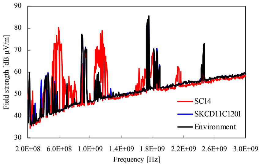
Figure 9: EMC measurement of helium-radiated device SC14 (impatt) and SKCD11C120I (no impatt) in comparison with environment
