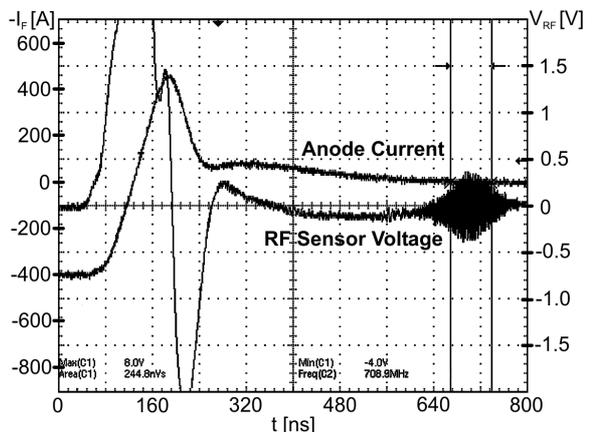
Figure 2: Measurement of a pett oscillation in a power module GAR with two paralleled diode chips
