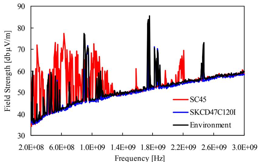
Figure 8: EMC measurement of electron-radiated device SC45 (impatt) and SKCD47C120I (no impatt) in comparison with environment
