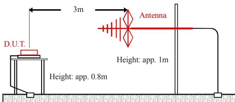
Figure 5: EMC measuring configuration
