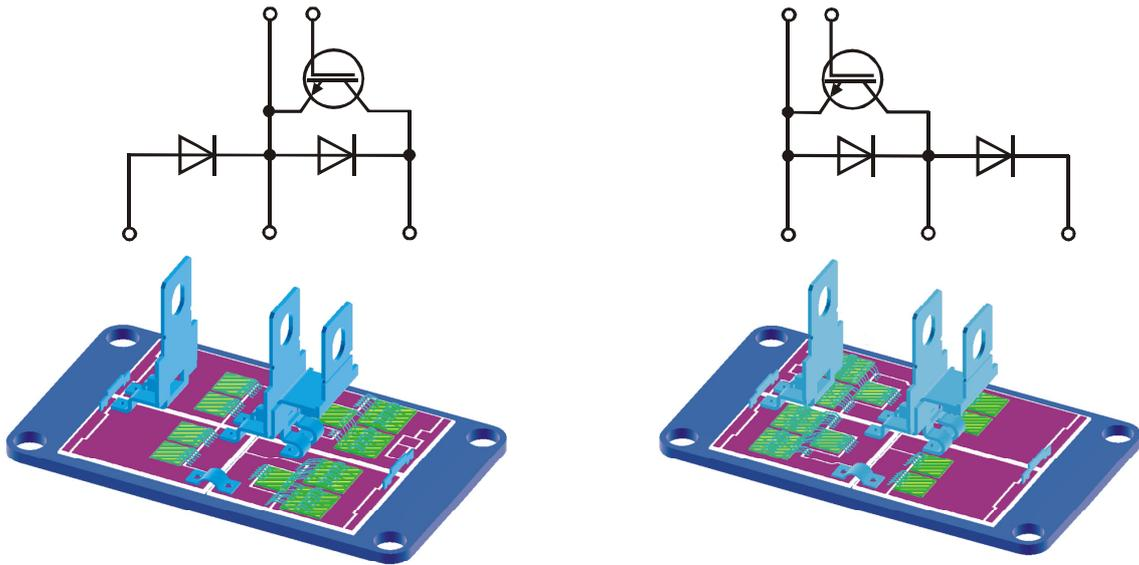
Figure 6: Internal circuit and module layout of high-side switch GAR (left) and low-side switch GAL (right)
