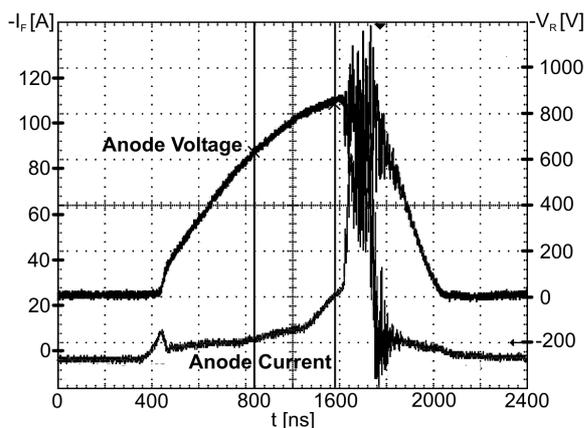
Figure 1: Measurement of a dynamic impatt oscillation at an electron-radiated freewheeling diode SC45
