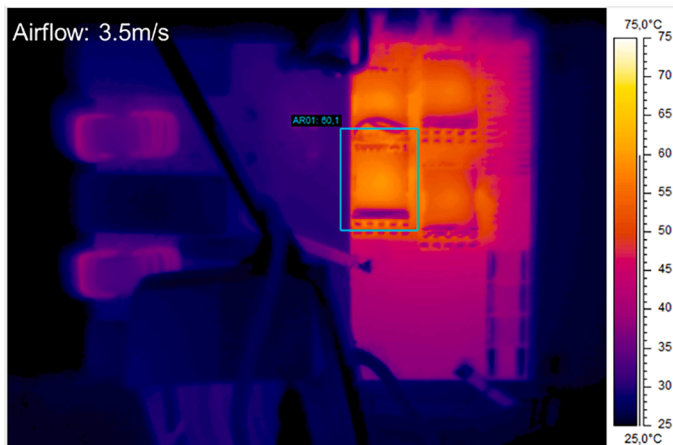
Fig. 22. Temperature distribution across the PFC module without heatsink [VAC = 230 V, VDC = 380 V, POUT = 1.6 kW].
