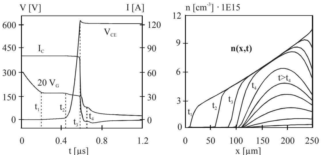
Figure 2: a) Turn-off characteristics
