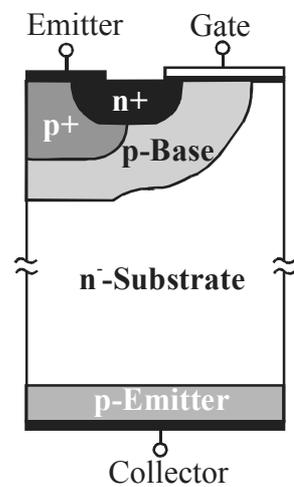
Figure 1: 1.2kV NPT IGBT
