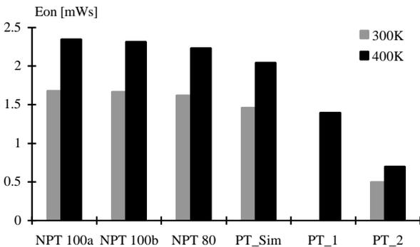
Figure 7: Comparison of IGBT turn-on losses at  $I_C=27A$
