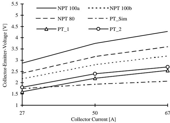
Figure 6: IGBT on-state characteristics at T=400K
