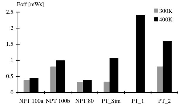
Figure 9: Comparison of IGBT turn-off losses at  $I_C=27A$
