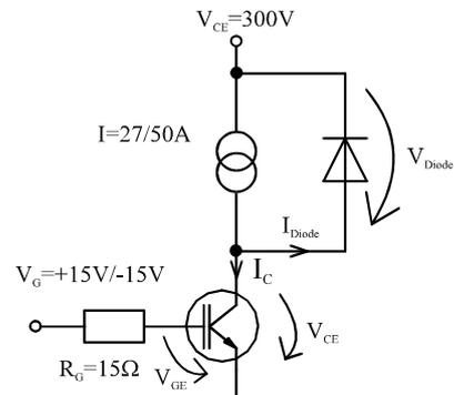
**Figure 2:** Schematic of the simulated circuit
