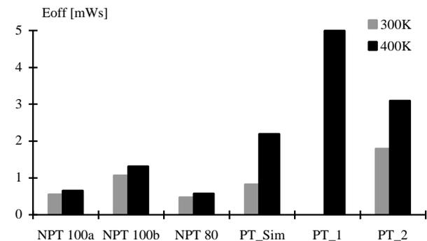
Figure 10: Comparison of IGBT turn-off losses at  $I_C=50A$
