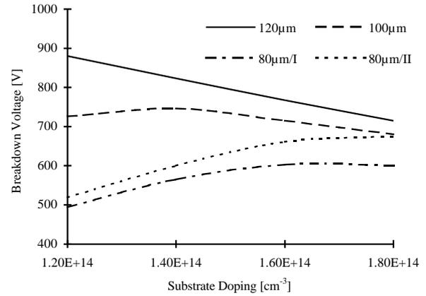
**Figure 4:** Breakdown voltage versus substrate doping (NPT-IGBT)
