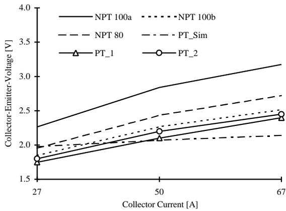
Figure 5: IGBT on-state characteristics at T=300K
