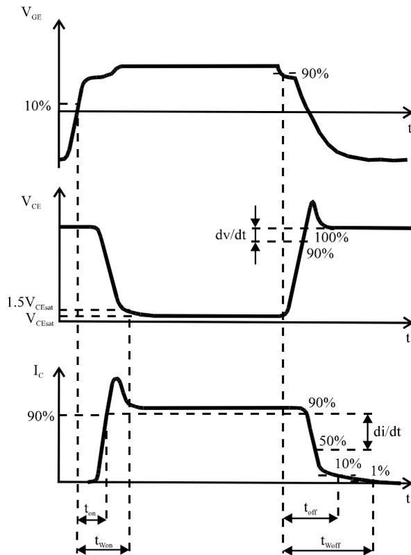
**Figure 3:** Definitions for device characterization
