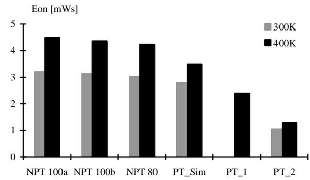
Figure 8: Comparison of IGBT turn-on losses at  $I_C=50A$
