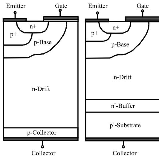
**Figure 1:** Structure of the NPT-IGBT(left) and the PT-IGBT(right)
