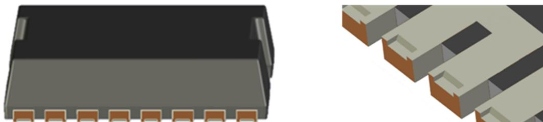
Fig. 10: Schematic view of the tinned grooves on the short leads
