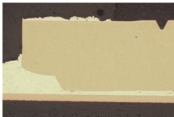
Fig. 12: Cross section through the soldered TO-Leadless device
