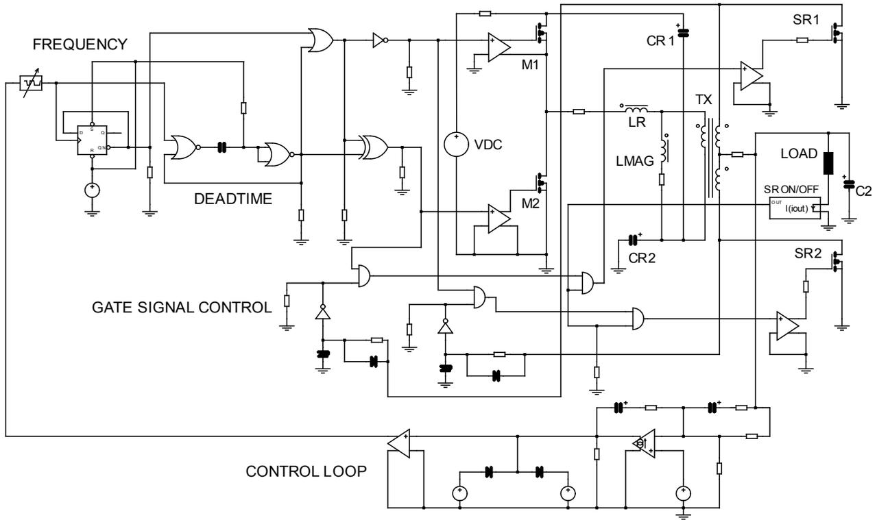
Fig. 12: Basic circuit simulation schematic representing the investigated LLC converter
