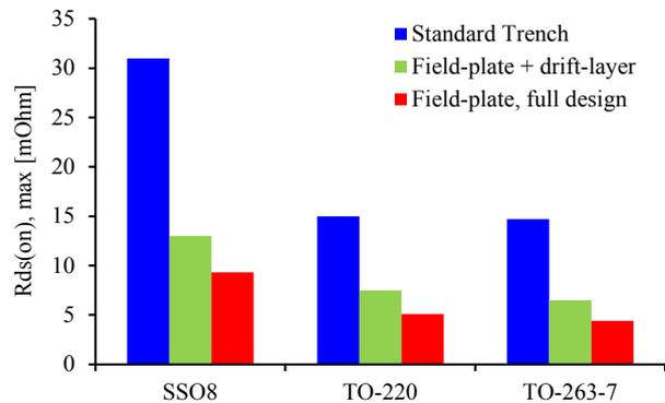
Fig. 8: Comparison of the product on-resistance of the 150 V devices with respect to the discussed concept approaches
