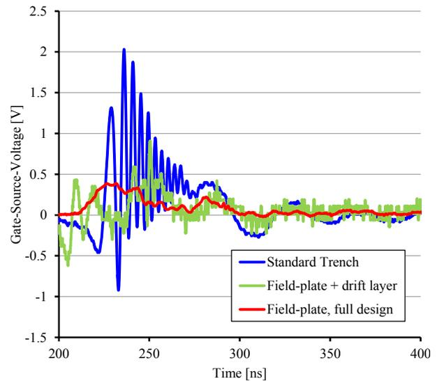
Fig. 19: Comparison of the SR-MOSFETs gate-to-source voltages during drain voltage upswing
