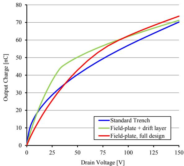
Fig. 10: Comparison of the output charge dependencies for an equivalent on-resistance of ca. 14 m $\Omega$
