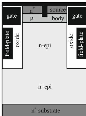
Fig. 6: Schematic cross section of a charge-compensated device with an additional drift layer
