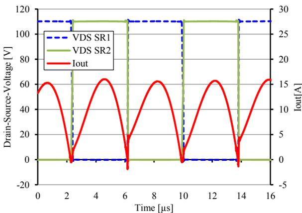
Fig. 13: Simulated waveforms for the drain-source voltage of the SR MOSFET and the rectified load current
