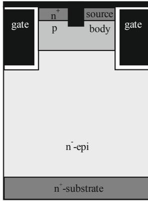
Fig. 5: Schematic cross section of a vertical trench power MOSFET
