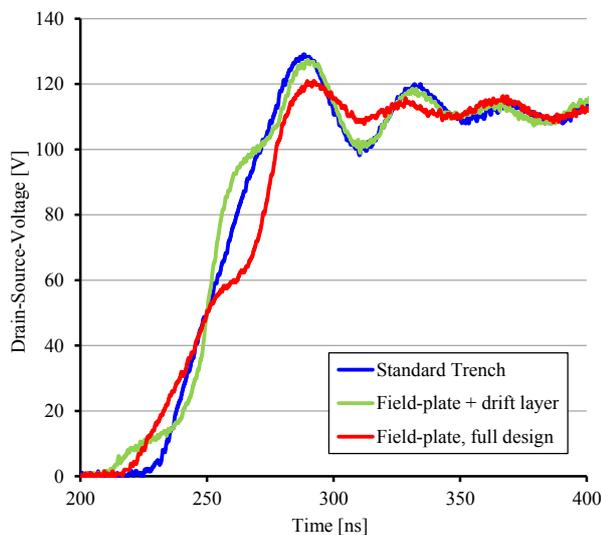
Fig. 18: Comparison of the SR-MOSFETs drain-to-source voltages during drain voltage upswing
