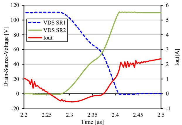
Fig. 14: Zoomed view into the drain-source voltage transition phase and the rectified load current
