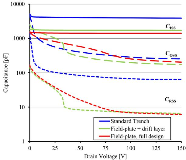
Fig. 9: Comparison of the input, output and reverse transfer capacitance for an equivalent on-resistance of ca. 14 m $\Omega$
