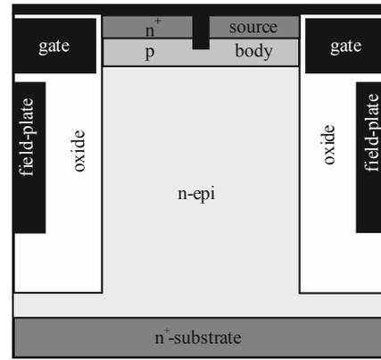
Fig. 7: Schematic cross section of a charge-compensated device designed for a higher blocking voltage
