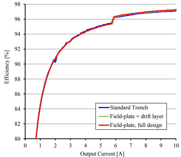
Fig. 16: Absolute converter efficiency comparison with respect to the different device technologies
