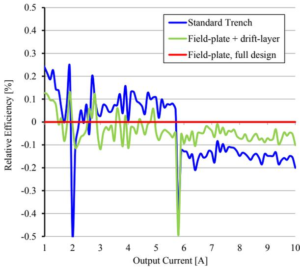
Fig. 17: Relative converter efficiency comparison with respect to the different device technologies
