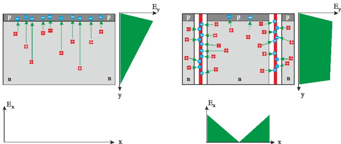
Fig. 4: Comparison of the electric field distribution for a simple pn-junction and for field-plate structure
