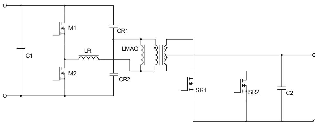
Fig. 1: Basic schematic of a LLC converter with synchronous rectification on the secondary side
