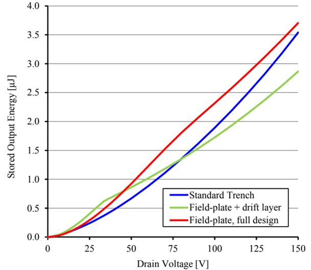
Fig. 11: Comparison of the stored output energy dependencies for an equivalent on-resistance of ca. 14 m $\Omega$
