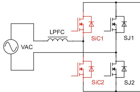
Fig. 4: Schematic of a full-bridge Totem Pole PFC
