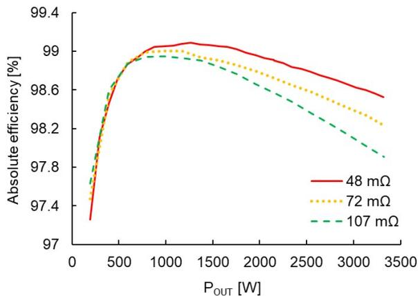
Fig. 15: Absolute efficiency at different  $R_{DS(on)}$  of 650 V SiC MOSFET in the CCM Totem Pole PFC
