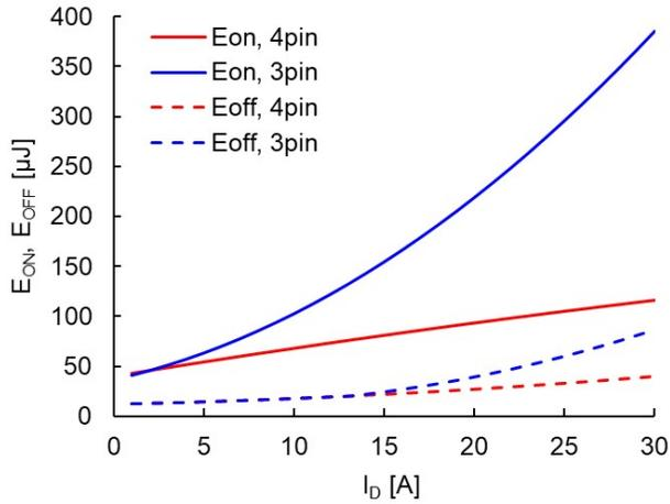
Fig. 11:  $E_{ON}$  (straight) and  $E_{OFF}$  (dashed) comparison TO-247 3pin (blue) vs. TO-247 4pin (red)
