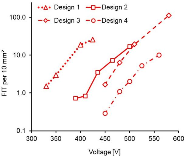
Fig. 7: Cosmic ray robustness of different designs
