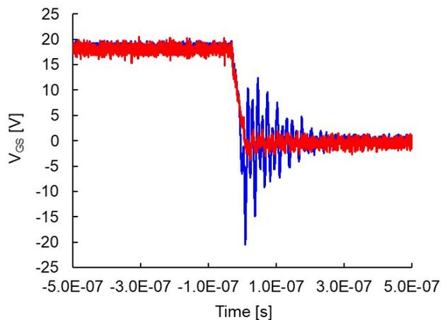
Fig. 13:  $V_{GS}$  at turn-off for TO-247 3pin (blue) vs. 4pin (red)
