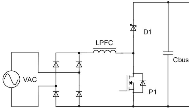
Fig. 2: Schematic of a typical Boost PFC stage
