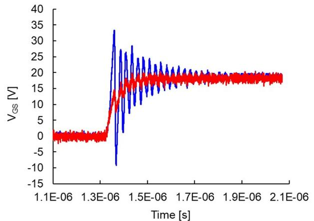
Fig. 12:  $V_{GS}$  at turn-on for TO-247 3pin (blue) vs. 4pin (red)
