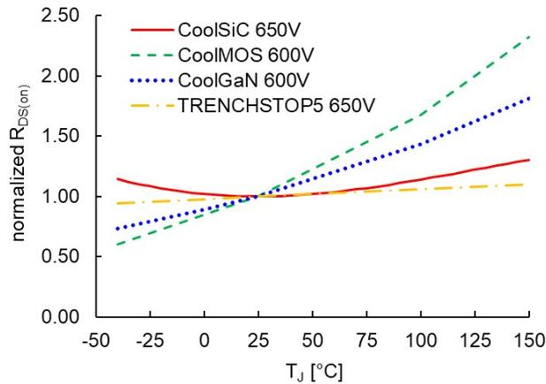
Fig. 14: Temperature dependence of normalized  $R_{DS(on)}$  for the different device technologies
