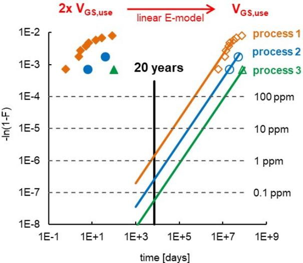
Fig. 6: Evaluation of on-state failure rate [8]
