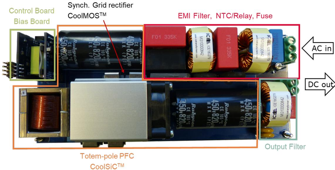
Fig. 8: The Totem Pole PFC test board
