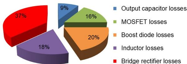
Fig. 1: Loss breakdown for a traditional Boost PFC
