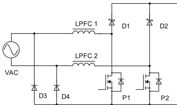
Fig. 3: Schematic of a Dual Boost PFC
