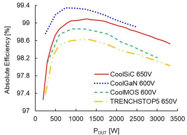
Fig. 16: Comparison of absolute efficiency of the different technologies
