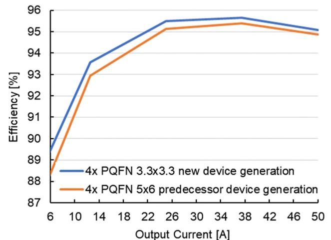
**Fig. 12** Comparison of the gained efficiency improvement in the 600 W IBC ( $V_{IN} = 54$  V)
