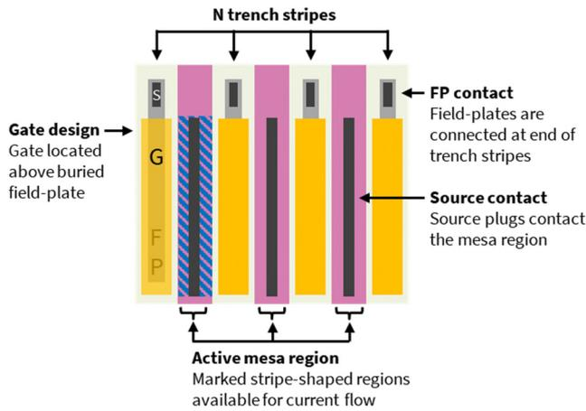
**Fig. 2** Typical Trench MOSFET with commonly employed stripe layout approach in the chip design
