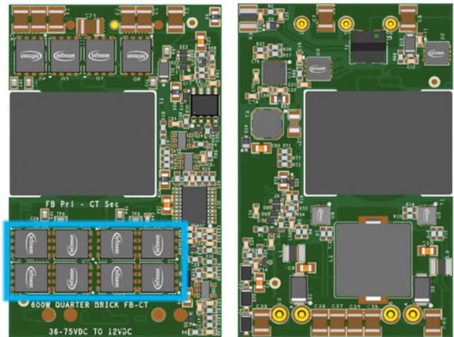
**Fig. 11** Top and bottom view of the 600 W IBC board with the secondary side MOSFET marked in blue
