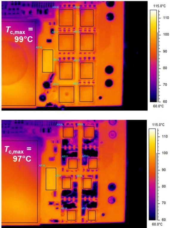
**Fig. 13** Temperature for the use of 4x PQFN 5x6 mm<sup>2</sup> devices of predecessor generation (top) with 4x PQFN 3.3x3.3mm<sup>2</sup> devices of the new generation (bottom)
