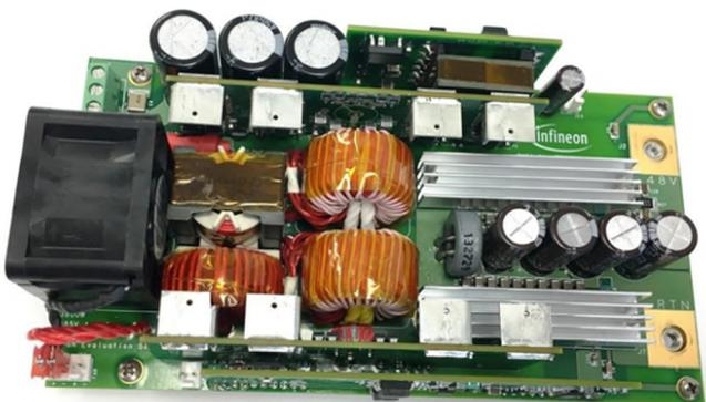
**Fig. 14** View of the employed 3.6 kW LLC DC-DC test board
