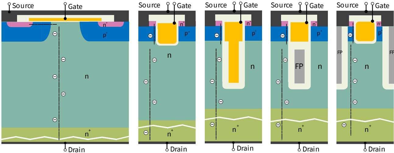
**Fig. 1** Exemplary device structures depicting the evolution of power MOSFET:
