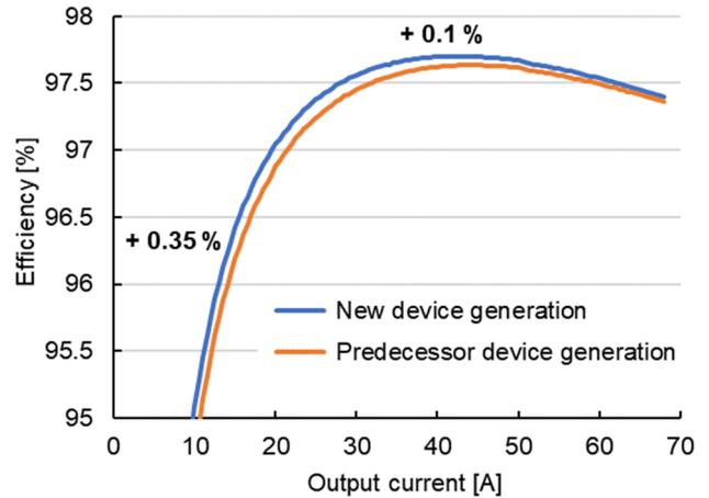
**Fig. 15** Comparison of gained efficiency in the 3.6 kW LLC DC-DC test board ( $V_{IN} = 385$  V,  $f_{SW} = 350$  kHz)
