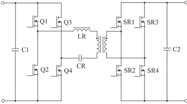
**Fig. 6** Basic schematic of the LLC DC-DC test boards
