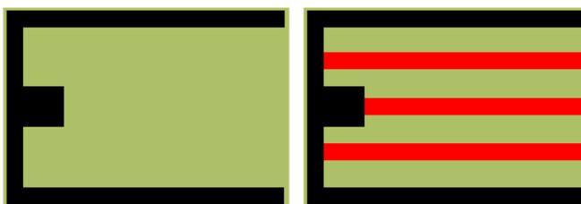
**Fig. 4** Illustration of active area loss on a MOSFET chip due to the introduction of gate fingers (red)
