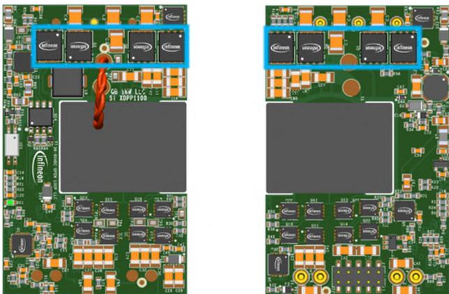
**Fig. 7** Top and bottom view of the 1 kW LLC DC-DC board with the primary side MOSFET marked in blue
