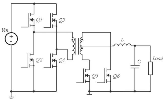
**Fig. 10** Basic schematic of the 600 W DC-DC IBC test board
