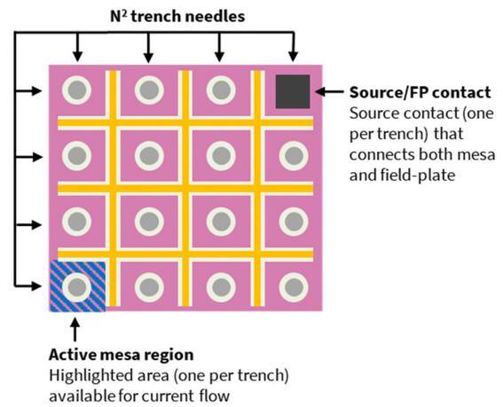
**Fig. 3** Trench MOSFET structure with the new grid-like layout approach in the new chip design
