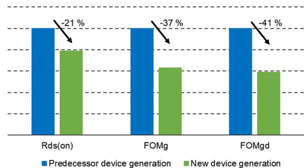
**Fig. 5** Gained improvements in device performance for a best-in-class 80 V device in PQFN 5x6 package
