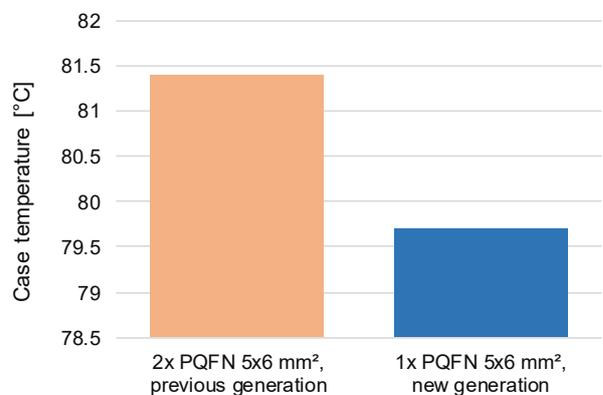
**Fig. 9** Case temperature for the different devices in the 1 kW LLC converter at maximum output current
