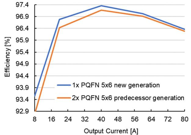
**Fig. 8** Comparison of the gained efficiency improvement in the 1 kW 4:1 LLC DC-DC converter ( $V_{IN} = 54$  V)
